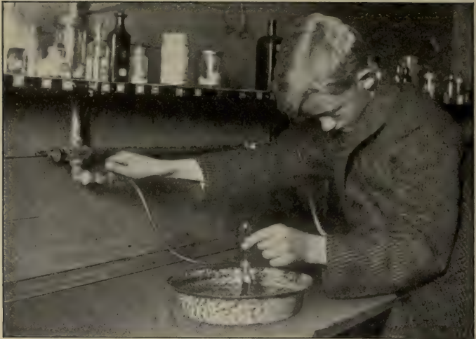
FIG. 149. Filling a test tube with gas.
